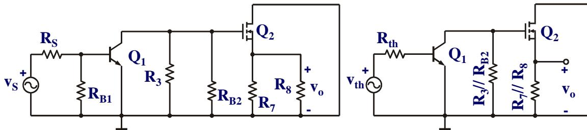
$$R_{B1} = R_1 // R_2 \quad R_{B2} = R_5 // R_6$$
